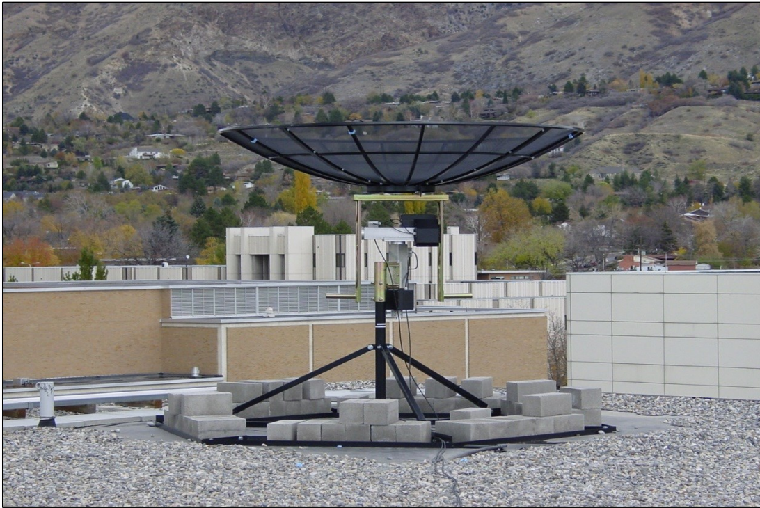
Figure 6-3: One of the VSA Antennas Located on The Engineering Clyde Building on the BYU Campus, shown with its mounting base, azimuth/elevation controller, counter weights, and base weights. Photo courtesy the BYU Electrical Engineering Research Group of Dr. Brian Jeffs and Dr. Karl Warnick.
