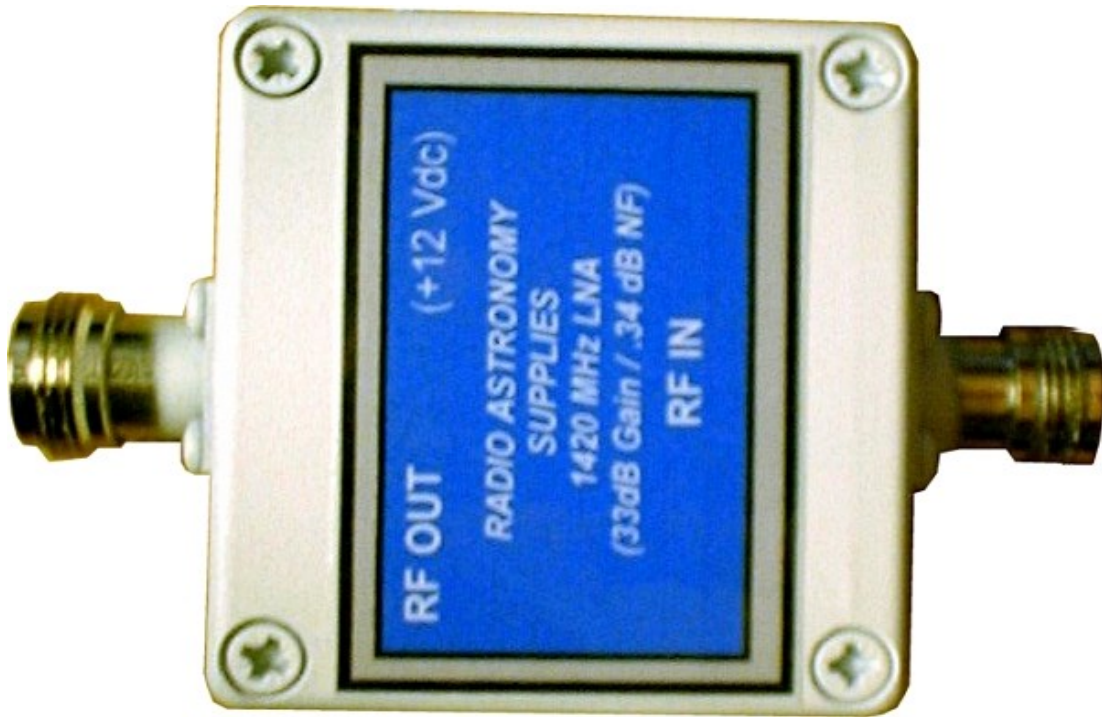
Figure 4-3: Radio Astronomy Supplies 1420 MHz LNA, having 33 dB gain at 0.34 dBm noise figure.
