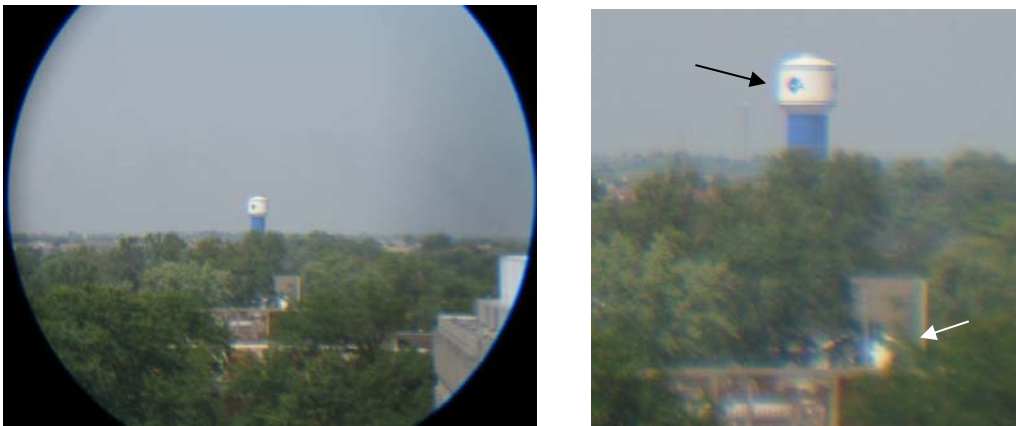
Fig.17 – The effects of chromatic and spherical aberration can be seen in these photographs taken through a small (1-inch aperture) non-achromatic telescope. Note the red and blue color fringes around bright objects, due to chromatic aberration, and the blurring, caused by spherical aberration (photographs by author)
