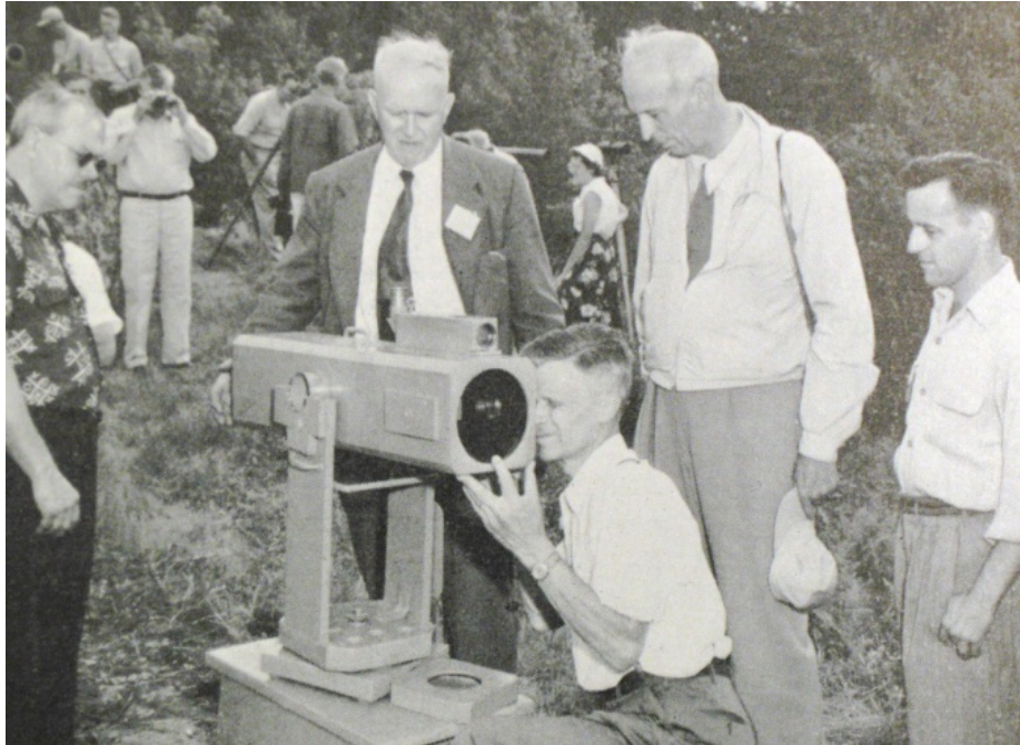
Fig. 52 – T. J. Ryan (far right) and interested spectators view his simply-mounted 6-inch f/5 Newtonian telescope at the 1954 Stellafane meeting (from Sky & Telescope ).
