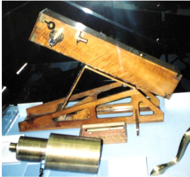
Fig. 22 – A Secrétaire-Foucault telescope with wooden tube and mount made around 1865 on display at the London Science Museum. The aperture is 10 cm (3.9 inches). The cylindrical brass object in the foreground is an eyepiece from Lord Rosse's 6-foot speculum-metal reflector (photograph by author).
